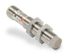
AutomationDirect capacitive proximity sensor, tubular, 12mm diameter x 61.2mm body, stainless steel housing, PNP, N.O. output, 12mm sensing distance, non-flush, 50 Hz switching frequency, IP65, 4-pin M12 quick-disconnect.
