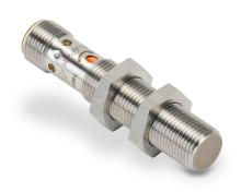
AutomationDirect capacitive proximity sensor, tubular, 12mm diameter x 59.8mm body, stainless steel housing, PNP, N.O. output, 6mm sensing distance, flush, 50 Hz switching frequency, IP65, 4-pin M12 quick-disconnect.
