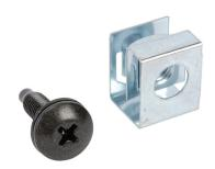
Hammond rack mounting screw, #10-32 UNF x 0.625in, #2 Phillips truss head, carbon steel, black oxide finish. Package of 50. Black nylon washer and zinc-plated clip nut included.
