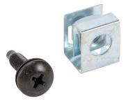
Hammond rack mounting screw, #10-32 UNF x 0.625in, #2 Phillips truss head, carbon steel, black oxide finish. Package of 25. Black nylon washer and zinc-plated clip nut included.
