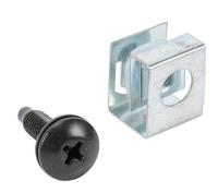
Hammond rack mounting screw, #10-32 UNF x 0.625in, #2 Phillips truss head, carbon steel, black oxide finish. Package of 100. Black nylon washer and zinc-plated clip nut included.
