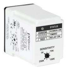
ProSense remote level controller, tank fill, (2) conductive level probes and (1) common probe input, (1) SPDT latching relay, fixed 1 second time delay output, 24 VAC operating voltage.
