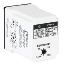
ProSense remote level controller, tank fill, (2) conductive level probes and (1) common probe input, (1) SPDT latching relay, fixed 1 second time delay output, 240 VAC operating voltage.
