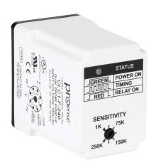
ProSense remote level controller, tank fill, (2) conductive level probes and (1) common probe input, (1) SPDT latching relay, fixed 1 second time delay output, 240 VAC operating voltage.
