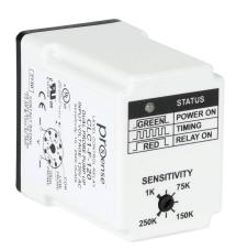
ProSense remote level controller, tank fill, (2) conductive level probes and (1) common probe input, (1) SPDT latching relay, fixed 1 second time delay output, 120 VAC operating voltage.
