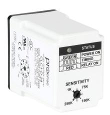
ProSense remote level controller, tank drain, (2) conductive level probes and (1) common probe input, (1) SPDT latching relay, fixed 1 second time delay output, 24 VAC operating voltage.
