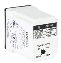
ProSense remote level controller, tank drain, (2) conductive level probes and (1) common probe input, (1) SPDT latching relay, fixed 1 second time delay output, 240 VAC operating voltage.
