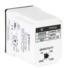
ProSense remote level controller, tank drain, (2) conductive level probes and (1) common probe input, (1) SPDT latching relay, fixed 1 second time delay output, 120 VAC operating voltage.
