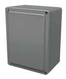
Stahlin Classic series enclosure, NEMA 1/3/3S/3R/4X/12,  $9 \times 7 \times 5$  in (HxWxD), wall mount, fiberglass reinforced polyester, gray, crowned hinged screw cover.
