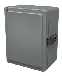
Stahlin Classic series enclosure, NEMA 1/3/3S/3R/4X/12, 9 x 7 x 5in (HxWxD), wall mount, fiberglass reinforced polyester, gray, crowned single-door, (1) quick-release latch, padlock hasp and staple.
