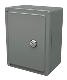
Stahlin Classic series enclosure, NEMA 1/3/3S/3R/4X/12,  $9 \times 7 \times 5$  in (HxWxD), wall mount, fiberglass reinforced polyester, gray, crowned single-door, (1) 1/4-turn flush-mounted latch.
