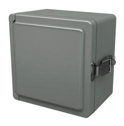
Stahlin Classic series enclosure, NEMA 1/3/3S/3R/4X/12,  $7 \times 7 \times 5$  in (HxWxD), wall mount, fiberglass reinforced polyester, gray, crowned single-door, (1) quick-release latch, padlock hasp and staple.
