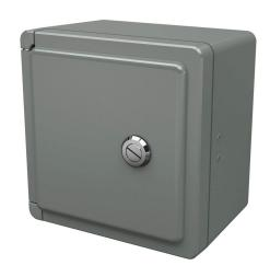
Stahlin Classic series enclosure, NEMA 1/3/3S/3R/4X/12,  $7 \times 7 \times 5$  in (HxWxD), wall mount, fiberglass reinforced polyester, gray, crowned single-door, (1) 1/4-turn flush-mounted latch.
