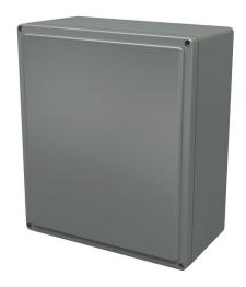
Stahlin Classic series enclosure, NEMA 1/3/3S/3R/4X/12, 15 x 13 x 7in (HxWxD), wall mount, fiberglass reinforced polyester, gray, crowned screw cover.
