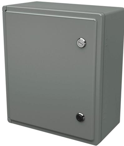
Stahlin Classic series enclosure, NEMA 1/3/3S/3R/4X/12, 15 x 13 x 7in (HxWxD), wall mount, fiberglass reinforced polyester, gray, crowned single-door, (1) 1/4-turn flush-mounted latch.
