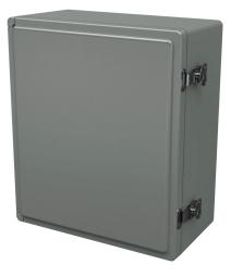
Stahlin Classic series enclosure, NEMA 1/3/3S/3R/4X/12, 15 x 13 x 7in (HxWxD), wall mount, fiberglass reinforced polyester, gray, crowned single-door, (2) twist-lock latches.
