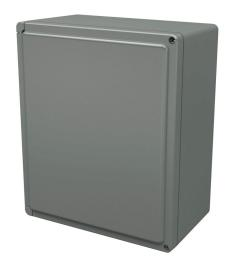
Stahlin Classic series enclosure, NEMA 1/3/3S/3R/4X/12, 13 x 11 x 6in (HxWxD), wall mount, fiberglass reinforced polyester, gray, crowned hinged screw cover.
