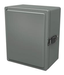
Stahlin Classic series enclosure, NEMA 1/3/3S/3R/4X/12,  $11 \times 9 \times 6$  in (HxWxD), wall mount, fiberglass reinforced polyester, gray, crowned single-door, (1) quick-release latch, padlock hasp and staple.
