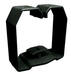
Iboco wire retainers, package of 20. For use with 2.25x2.25in duct. Fastens to duct with integral twist fasteners.
