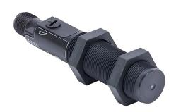
AutomationDirect capacitive proximity sensor, tubular, 18mm diameter x 92.5mm body, polybutylene terephthalate housing, PNP, N.C. output, 15mm sensing distance, non-flush, 30 Hz switching frequency, IP65 IP67 IP69K, 4-pin M12 quick-disconnect.
