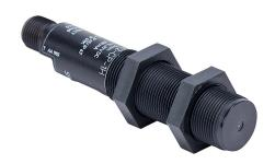
AutomationDirect capacitive proximity sensor, tubular, 18mm diameter x 92.5mm body, polybutylene terephthalate housing, PNP, N.C. output, 8mm sensing distance, flush, 30 Hz switching frequency, IP65 IP67 IP69K, 4-pin M12 quick-disconnect.
