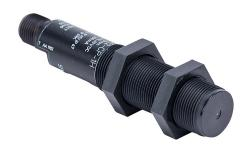
AutomationDirect capacitive proximity sensor, tubular, 18mm diameter x 92.5mm body, polybutylene terephthalate housing, PNP, N.C. output, 8mm sensing distance, flush, 30 Hz switching frequency, IP65 IP67 IP69K, 4-pin M12 quick-disconnect.
