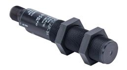
AutomationDirect capacitive proximity sensor, tubular, 18mm diameter x 92.5mm body, polybutylene terephthalate housing, PNP, N.O. output, 8mm sensing distance, flush, 30 Hz switching frequency, IP65 IP67 IP69K, 4-pin M12 quick-disconnect.
