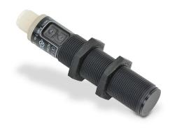
AutomationDirect capacitive proximity sensor, tubular, 18mm diameter x 87mm body, polybutylene terephthalate housing, NPN/PNP, N.O./N.C. selectable output, 12mm sensing distance, non-flush, 10 Hz switching frequency, IP65 IP67, 4-pin M12 quickdisconnect.
