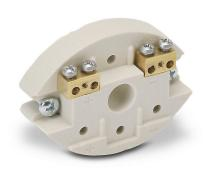
ProSense terminal base, (2) brass terminals with stainless steel screws, ceramic. For use with ProSense temperature probe connection heads.
