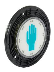
Captron capacitive pushbutton sensor switch, IP69K, 60mm, dynamic, polycarbonate bezel, semi-automatic LED control, Operator: white, 100mm, operator text "hand symbol", green. Requires 4-pin female M8 cable and AR4 cover ring.
