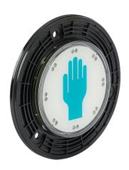
Captron capacitive pushbutton sensor switch, IP69K, 60mm, dynamic, polycarbonate bezel, manual LED control, Operator: white, 100mm, operator text "hand symbol", green. Requires 5-pin female M8 cable and AR4 cover ring.
