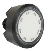
Captron capacitive pushbutton sensor switch, IP69K, 22mm, static, Delrin bezel, semi-automatic LED control, Operator: white, 60mm. Requires 4-pin female M8 cable.
