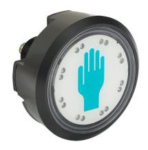
Captron capacitive pushbutton sensor switch, IP69K, 22mm, dynamic, Delrin bezel, manual LED control, Operator: white, 60mm, operator text "hand symbol", green. Requires 5-pin female M8 cable.
