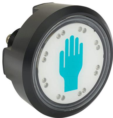
Captron capacitive pushbutton sensor switch, IP69K, 22mm, static, Delrin bezel, manual LED control, Operator: white, 60mm, operator text "hand symbol", green. Requires 5-pin female M8 cable.
