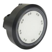
Captron capacitive pushbutton sensor switch, IP69K, 22mm, dynamic, Delrin bezel, manual LED control, Operator: white, 60mm. Requires 5-pin female M8 cable.
