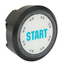
Captron capacitive pushbutton sensor switch, IP69K, 22mm, static, Delrin bezel, manual LED control, Operator: white, 60mm, operator text "START", green. Requires 5-pin female M8 cable.
