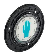
Captron capacitive pushbutton sensor switch, IP69K, 50mm, dynamic, polycarbonate bezel, semi-automatic LED control, Operator: white, 88mm, operator text "hand symbol", green. Requires 4-pin female M8 cable and AR3 cover ring.
