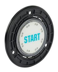
Captron capacitive pushbutton sensor switch, IP69K, 50mm, static, polycarbonate bezel, semi-automatic LED control, Operator: white, 88mm, operator text "START", green. Requires 4-pin female M8 cable and AR3 cover ring.
