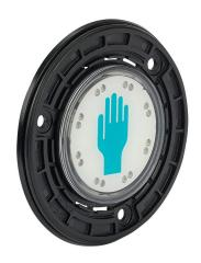
Captron capacitive pushbutton sensor switch, IP69K, 50mm, dynamic, polycarbonate bezel, manual LED control, Operator: white, 88mm, operator text "hand symbol", green. Requires 5-pin female M8 cable and AR3 cover ring.
