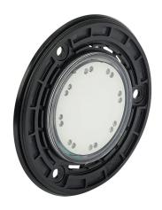
Captron capacitive pushbutton sensor switch, IP69K, 50mm, dynamic, polycarbonate bezel, manual LED control, Operator: white, 88mm. Requires 5-pin female M8 cable and AR3 cover ring.
