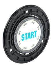
Captron capacitive pushbutton sensor switch, IP69K, 50mm, dynamic, polycarbonate bezel, manual LED control, Operator: white, 88mm, operator text "START", green. Requires 5-pin female M8 cable and AR3 cover ring.
