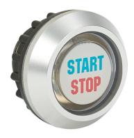
Captron capacitive pushbutton sensor switch, IP69K, 22mm, toggle, aluminum bezel, semi-automatic LED control, Operator: white, 28.5mm, operator text "START/STOP", green and red. Requires 4-pin female M8 cable.
