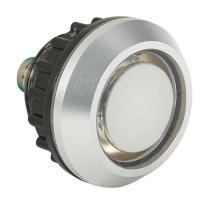
Captron capacitive pushbutton sensor switch, IP69K, 22mm, toggle, aluminum bezel, semi-automatic LED control, Operator: white, 28.5mm. Requires 4-pin female M8 cable.
