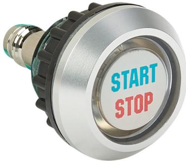
Captron capacitive pushbutton sensor switch, IP69K, 22mm, toggle, aluminum bezel, manual LED control, Operator: white, 28.5mm, operator text "START/STOP", green and red. Requires 5-pin female M8 cable.
