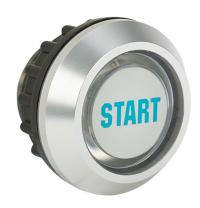
Captron capacitive pushbutton sensor switch, IP69K, 22mm, static, aluminum bezel, semi-automatic LED control, Operator: white, 28.5mm, operator text "START", green. Requires 4-pin female M8 cable.
