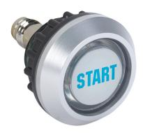
Captron capacitive pushbutton sensor switch, IP69K, 22mm, static, aluminum bezel, manual LED control, Operator: white, 28.5mm, operator text "START", green. Requires 5-pin female M8 cable.
