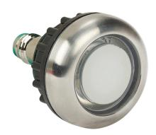
Captron capacitive pushbutton sensor switch, IP69K, 22mm, static, stainless steel bezel, manual LED control, Operator: white, 28.5mm. Requires 5-pin female M8 cable.
