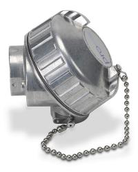
ProSense general purpose screw cover connection head, 1/2in female NPT probe connection, 3/4in female NPT conduit opening, maximum temperature rating of 825 deg F (440 deg C), die-cast aluminum, NEMA 4X, IP66.
