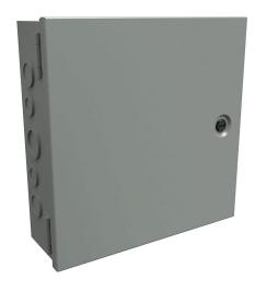
Hammond enclosure, NEMA 1, 8 x 8 x 6in (HxWxD), wall mount, with knockouts, carbon steel, ANSI 61 gray, powder coat finish, single-door, 1/4-turn flush-mounted latch.
