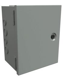
Hammond enclosure, NEMA 1, 6 x 6 x 6 in (HxWxD), wall mount, with knockouts, carbon steel, ANSI 61 gray, powder coat finish, single-door, 1/4-turn flush-mounted latch.
