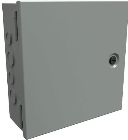
Hammond enclosure, NEMA 1, 6 x 4 x 4in (HxWxD), wall mount, with knockouts, carbon steel, ANSI 61 gray, powder coat finish, single-door, 1/4-turn flush-mounted latch.
