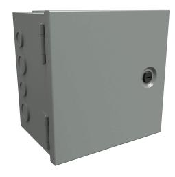
Hammond enclosure, NEMA 1, 36 x 24 x 8in (HxWxD), wall mount, with knockouts, carbon steel, ANSI 61 gray, powder coat finish, single-door, 1/4-turn flush-mounted latch.
